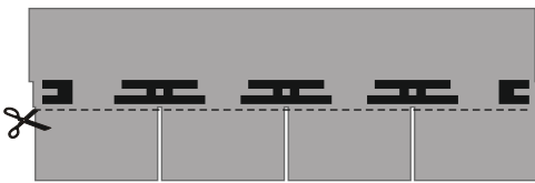
Fig. 2 Trimming the tabs
