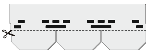
Fig. 2 Trimming the tabs
